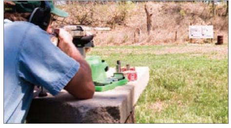
Shooting from a rest allows Scott to determine the effectiveness of the choke and load and also tells him about the gun's point of impact.
