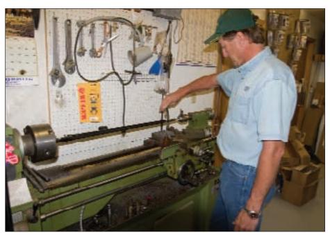
Scott reams a fixed choke barrel to prepare it for screw-in chokes. Custom screw-in choke tubes can make your favorite fixed-choke shotgun much more versatile.
