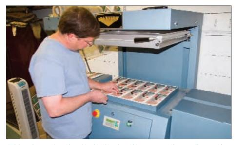
Choke tubes aren't machined at the shop, but all are measured for specifications, then laser labeled and packaged. Larry Allahman operates the shrink-wrap package machine above. Carlson's chokes are sold in the U.S., Canada, Greece, Australia, and England.
